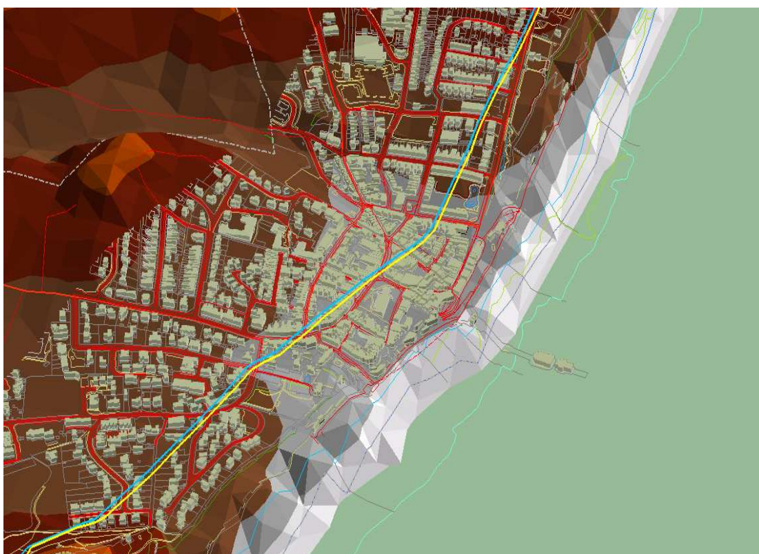
Fig. 6. An example of estimated cliff-top retreat for 2100 showing both recession lines (under scenario 43 – see Table 1). Land seaward of the right hand (yellow) line is assumed to be lost, while land between the two lines is at risk.
